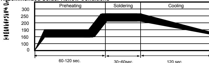
• Recommended reflow methods : IR, vapor phase oven, hot air oven.
