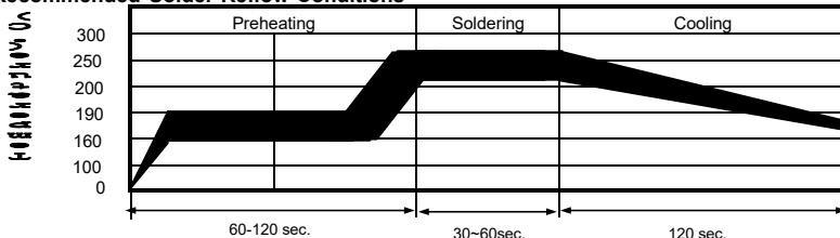
Recommended reflow methods: IR, vapor phase oven, hot air oven.
