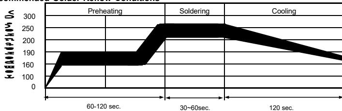
Recommended reflow methods: IR, vapor phase oven, hot air oven.
